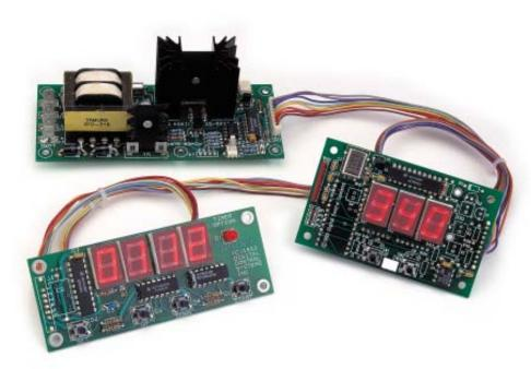
Designed for equipment manufacturers, the Model 120 provides a cost-effective way to quickly and simply incorporate state-of-the-art microprocessor-based control capabilities into a wide variety of products. It accurately regulates electrically controlled thermal processes operating at temperatures between 0 and 400 degrees Celsius, typically maintaining temperature stability to within one degree of setpoint.
