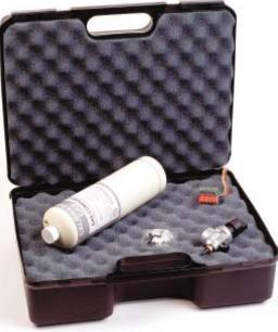
Created for the HVAC professional, the AirSense Calibration Kit is convenient, complete and sturdy. Housed in a compact, heavy duty carrying case, this calibration kit can safely travel from one installation to another or between job sites in the back of your truck. It contains the precise gas(es) and accessories you need to accurately calibrate your monitoring instruments.
