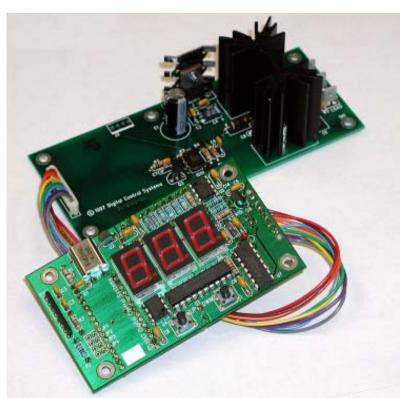
Designed for manufacturers of vehicular or other low voltage DC powered equipment, the Model 105 provides a cost-effective way to quickly and simply incorporate state of the art microprocessor based control capabilities into a wide variety of products. It precisely regulates electrically controlled thermal processes operating at temperatures between -9.9 and 99.9 degrees Celsius, typically maintaining temperature stability to well within  $\pm 0.1$  degrees of setpoint.
